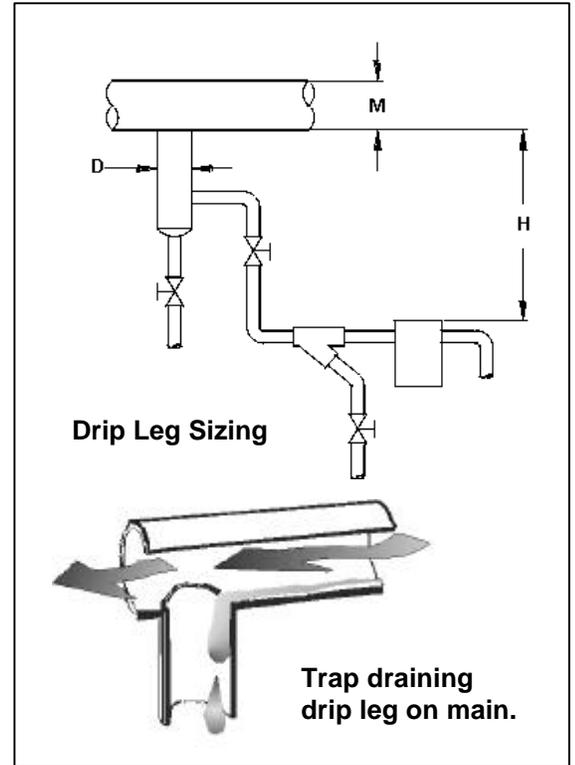
The question arises on whether insulation should be used on the drip leg, piping leading to the trap, and the trap. The answer is no; unless it is mandatory for safety reasons, this section of the steam system should not be insulated. The reason for this is to ensure that some condensate is continuously being formed ahead of the trap. This will ensure that the trap has some condensate going to it at all times, thus prolonging the trap's life.
