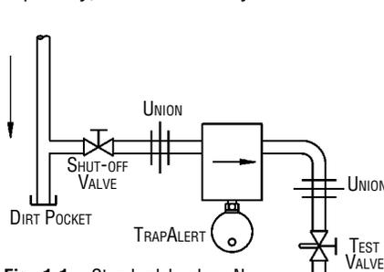
**Fig. 1-1.** Standard hookup No. 800-816, 880-883 traps, with shutoff valves to isolate trap during testing, inspection or repair. Unions should be at right angles—not inline—to facilitate trap removal.
