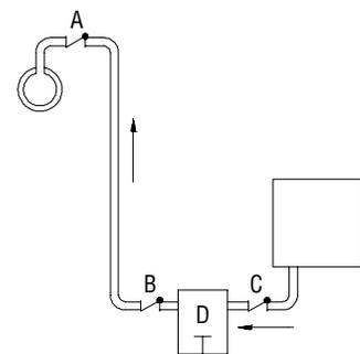
**Fig. 1-8.** Possible check valve locations.
