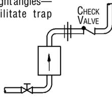
**Fig. 1-3.** No. 880-883 with strainer blowdown valve.
