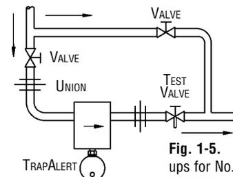
**Fig. 1-5.** Bypass hookups for No. 800-816 and 880-883 traps.
