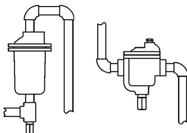
Fig. 2-5. Traps installed with short, well pitched discharge lines to prevent freezeups.
