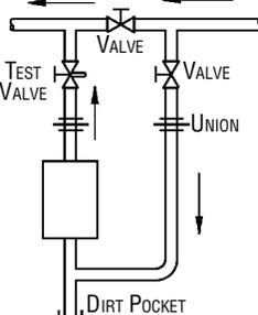
**Fig. 1-6.** Bypass hookup for No. 211-216 & 411 traps.
