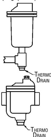
Fig. 2-2. 200 Series trap with Thermo Drain in tee ahead of trap. **Trap inlet tube must be removed.**
