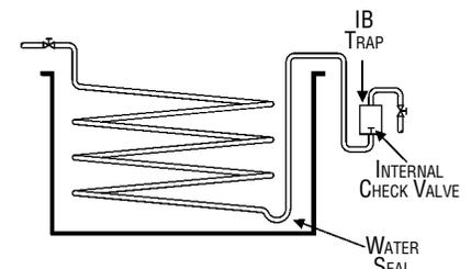
**Fig. 1-7.** Trap draining syphon.
