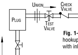
**Fig. 1-4.** Alternate hookup for No. 800-816 with inlet at bottom.
