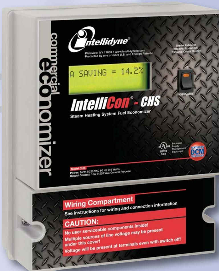
**IntelliCon<sup>®</sup>-CHS** is a microprocessor-based, fuel-saving control for commercial steam heating systems. *IntelliCon-CHS* reduces: fuel consumption, wear on parts, flue emissions and electrical usage when installed on any new or existing gas or oil burner. *IntelliCon-CHS* uses intelligent Dynamic Cycle Management (DCM) technology to save energy by adjusting the burner run pattern to match the system's "heat load."
